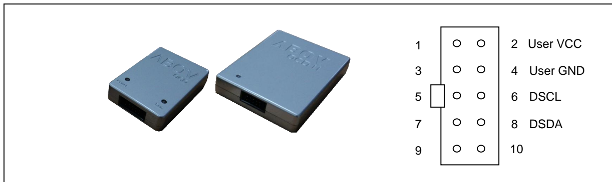
Figure 1.1 Debugger(OCD1/OCD2) and Pin description
